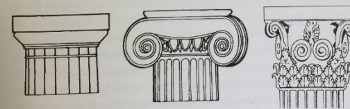
32. Greek architectural orders. Drawing of column capitals (left to right): Doric, Ionic, Corinthian.
