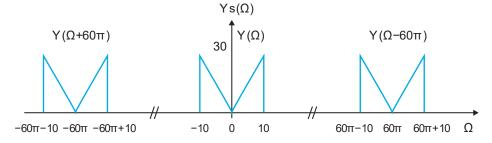
We note that there is sufficient empty spectral space between spectrum repetitions (due to sampling) so that the spectra do not overlap. We can easily recover the original signal by filtering the above spectrum with a deep-pass filter with a cutoff frequency that satisfies the equation:  $10 < \Omega_c < 60\pi - 10$ .
