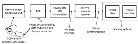
Figure 2.4 The processing components of the artificial retina (Schwiebert et al. 2001)
