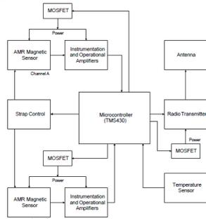
Figure 2.3 Block diagram of the MIT node for traffic monitoring (Knaian 2000)
