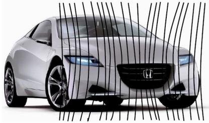
Figure 2.2 Detection of a moving vehicle with an ARM magnetic sensor (Caruso and Withanawasam 1999)
