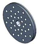
Create the WHEEL part with the Extruded Boss/Base feature on tool. Utilize the Mid Plane option to center the WHEEL on the Front Plane.
