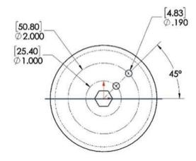
Sketch two additional Construction line bolt circles, 1.500in, [38.1] and 2.500in, [63.5]. Create the first Construction bolt circle.
