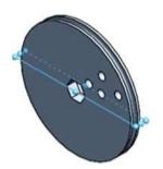
Utilize the Circular Pattern Feature tool. The two Extruded Cut features are contained in the Circular Pattern. Revolve the Extruded Cut features about the Temporary Axis located at the center of the Hexagon.
