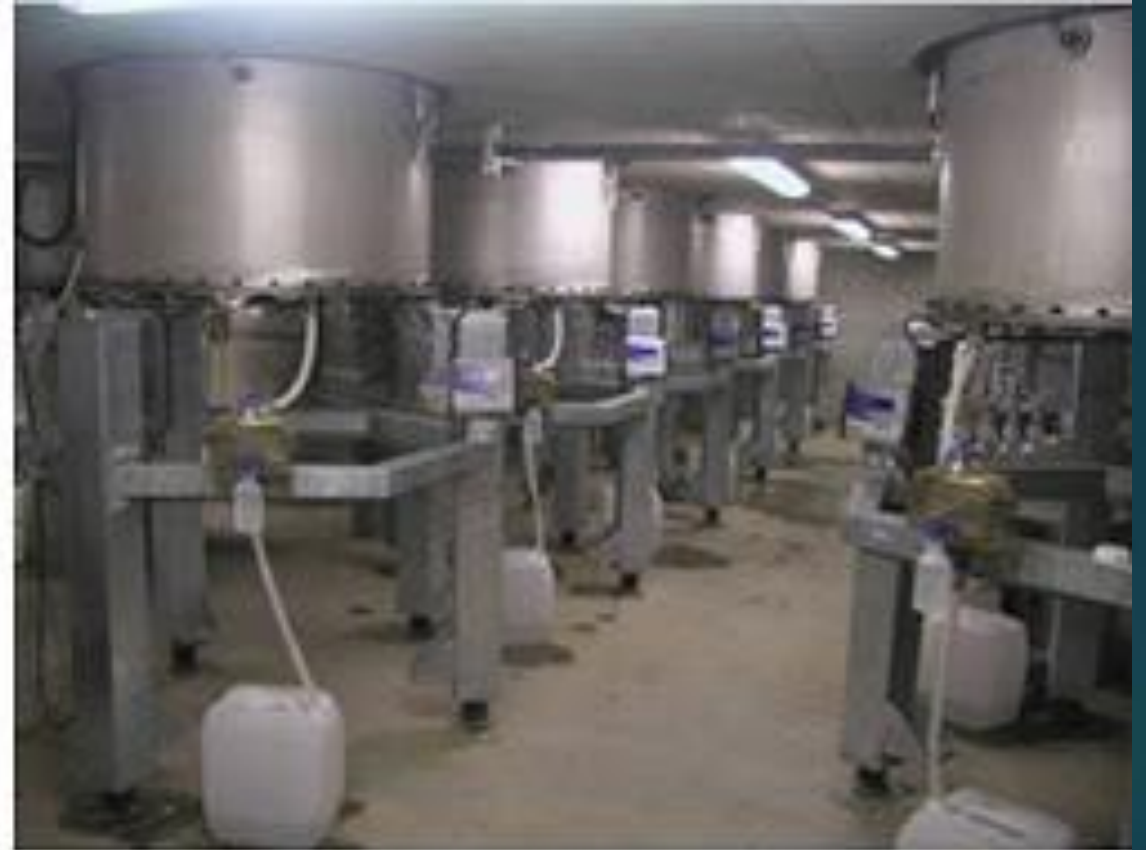
Figure 3. Above ground and below ground view of a weighing lysimeter.
