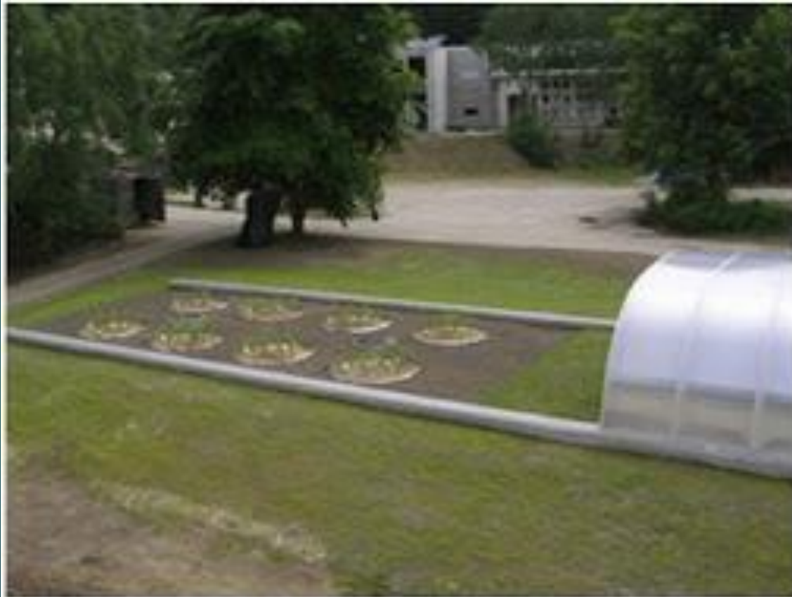
Figure 3. Above ground and below ground view of a weighing lysimeter.
