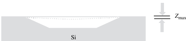
Figure 4.6 Basic MEMS pressure transducer.
