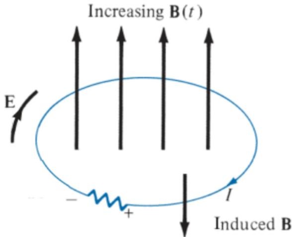
$$V_{\text{emf}} = \oint_L \mathbf{E} \cdot d\mathbf{l} = - \int_S \frac{\partial \mathbf{B}}{\partial t} \cdot d\mathbf{S} = \int_S (\nabla \times \mathbf{E}) \cdot d\mathbf{S} \Rightarrow \nabla \times \mathbf{E} = - \frac{\partial \mathbf{B}}{\partial t} \neq 0$$
