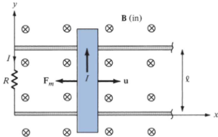
$$\mathbf{F}_m = I\mathbf{l} \times \mathbf{B} \Rightarrow F_m = I\ell B \quad \text{και} \quad V_{\text{emf}} = uB\ell$$
