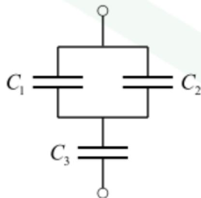
View the capacitor as a series/parallel combination of capacitors.
