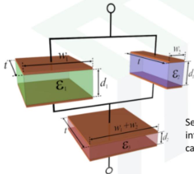
Separate the inhomogeneous capacitor into a combination of homogeneous capacitors.
