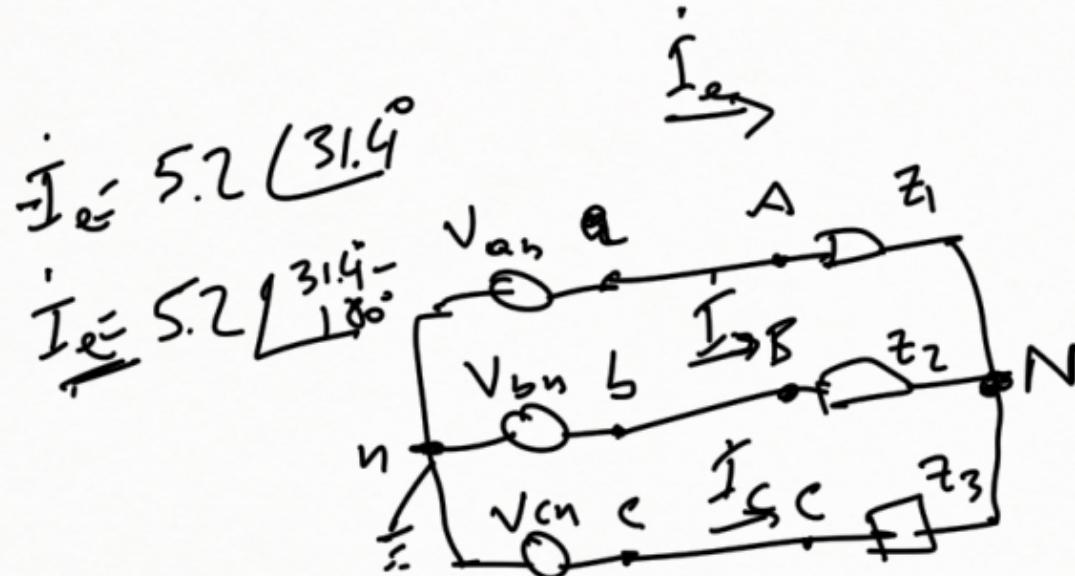
$$\dot{V}_N = \frac{\dot{V}_{an}}{z_1} + \frac{\dot{V}_{bn}}{z_2} + \frac{\dot{V}_{cn}}{z_3}$$
