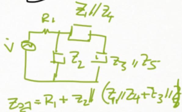
$$Z_{22} = R_1 + Z_2 \parallel (Z_1 \parallel Z_4 + Z_3 \parallel Z_5)$$
