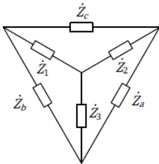
$$\dot{Z}_a = \frac{\dot{Z}_1 \dot{Z}_2 + \dot{Z}_2 \dot{Z}_3 + \dot{Z}_3 \dot{Z}_1}{\dot{Z}_1}$$
