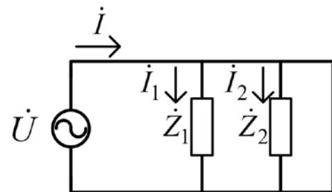
$$\dot{Z} = \frac{1}{\frac{1}{\dot{Z}_1} + \frac{1}{\dot{Z}_2}} = \frac{\dot{Z}_1 \dot{Z}_2}{\dot{Z}_1 + \dot{Z}_2}$$
